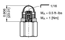
Air bleeding with capped adjustment screw "B"
