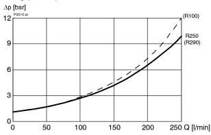
$\Delta p$  = f (Q) Pressure drop - Flow rate characteristic Lowering ( B  $\rightarrow$  A, spool fully open)
