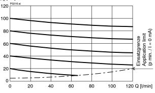
p = f (Q) Pressure - Flow rate characteristic  $p_{N}$  = 250 bar  $_{P_{A}\left[ bar \right] }$
