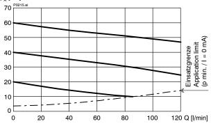
p = f (Q) Pressure - Flow rate characteristic  $p_N$  = 160 bar  $_{p_A}$  [bar]
