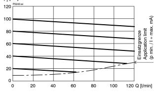
p = f (Q) Pressure - Flow rate characteristic  $\ p_{N}$  = 230 bar  $_{p_{2}}\left[ \text{bar} \right]$
