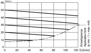
p = f (Q) Pressure - Flow rate characteristic  $\ p_{N}$  = 160 bar  $_{p_{2}}\left[ \mathsf{bar}\right]$
