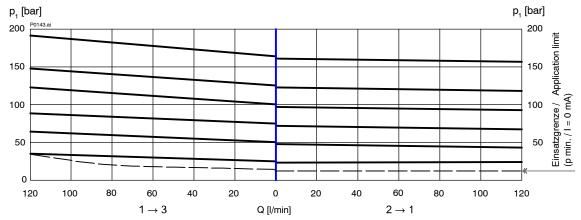
p = f(Q) Pressure - Flow rate characteristic [ $p_N = 250$  bar]
