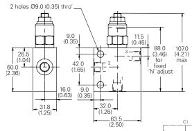
Double Valve with Housing **Basic Code** 1CEE34
