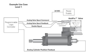
AxisPro level 1 KBH valves, can be used to control machine motions in open loop or closed loop control applications. The valve receives its analog command input on the 7-pin, main, connector from an external axis control device.
