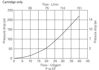
Note: Minimum inlet flow should not be less than 1/4 of maximum inlet flow. Minimum pressure drop is determined by control pressure.
